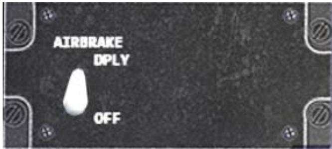
Fig 1: Air brake panel.
