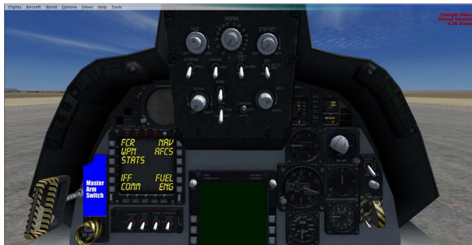
Fig 2. Master Arm Switch Location
