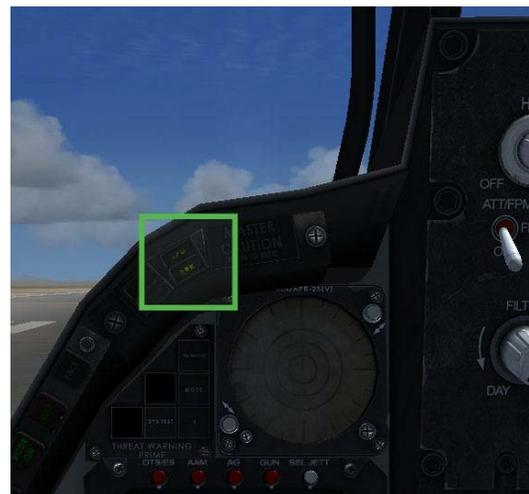
Fig. 3: Air brake Warning Light.
