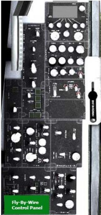
Fig 2: FBW Control Panel Location.
