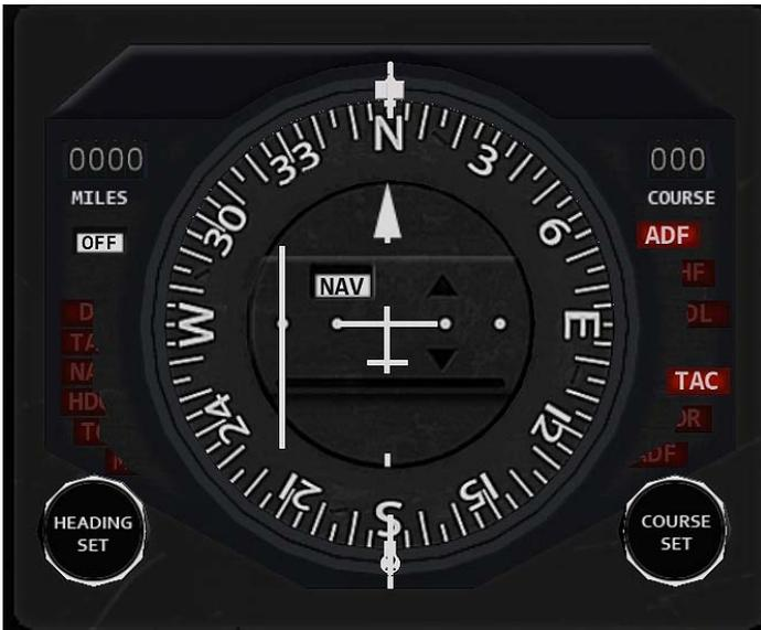
Fig. 1: The Horizontal Situation Indicator (HSI)
