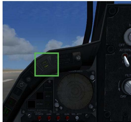
Fig. 3: Air brake Warning Light.
