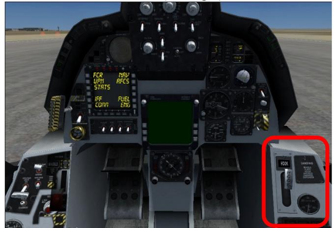
Fig 2: Arresting Hook Lever Location
