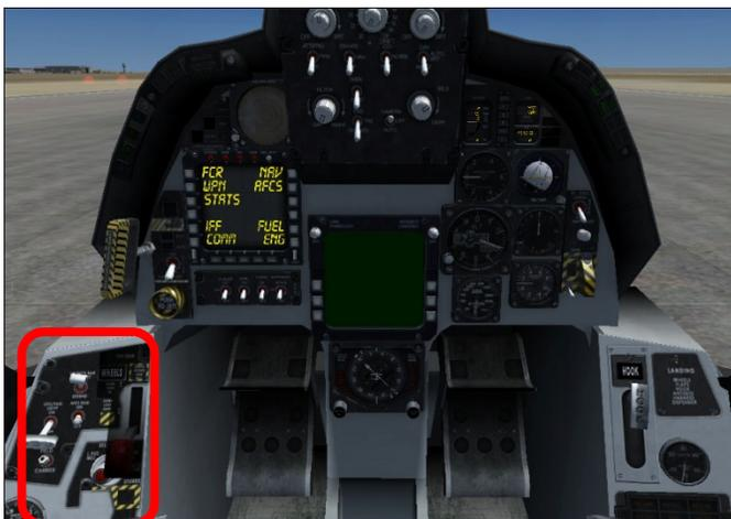
Fig 2: Landing Gear Panel Location
