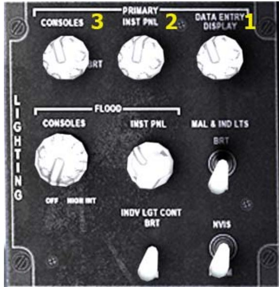
Fig 1: Internal Lights Panel
