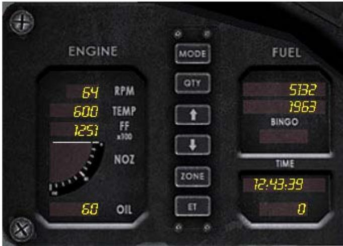
On the Upper Right section of the main instrument panel, just besides the HUD control panel an Auxiliary ENGINE/FUEL Panel can be seen.
