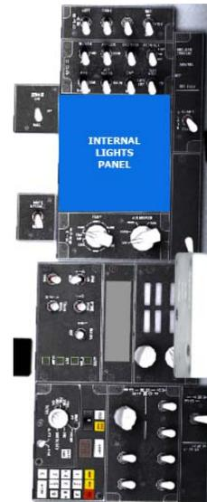
Fig 4: Internal Lights Panel Location.
