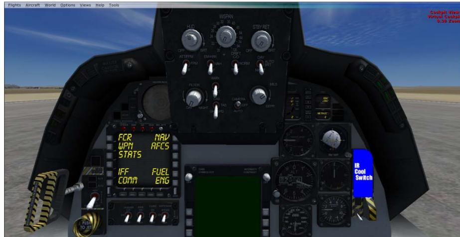
Fig 2. IR Cool Switch Location
