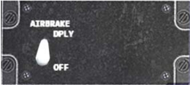
Fig 1: Air brake panel.
