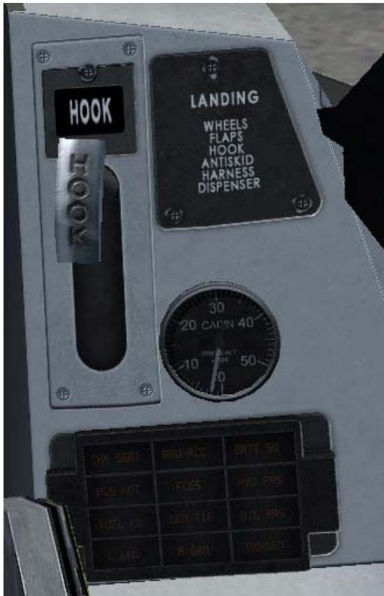
Fig 1: Arresting Hook Lever
